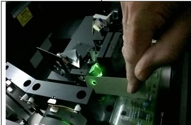
Light passing in direction of the mirror will be reflected and will hit again the paper: if the reflected light is not superimposed with the hole (i.e. if a bright halo is visible around the hole) then the instrument is slightly misaligned.
