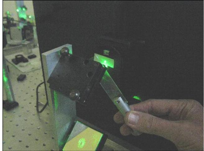
Caution: do not rotate the glass plate too far or the scattered light beam will be displaced so that it does not enter the pinhole. If the light does not go in, it cannot come out again!
